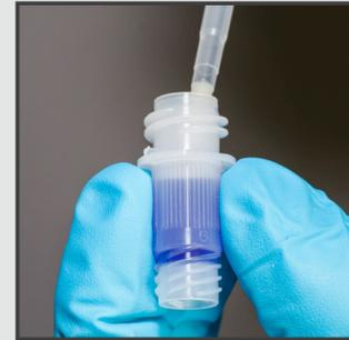
> Transfer the sample slowly into the heating tube. Slowly rinse the tip once to remove the sputum.
