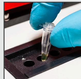
> Incubate the reaction tube at 67°C for 40 min in the reaction unit. The reaction is automatically inactivated by a further incubation step at 80°C for 5 min.
