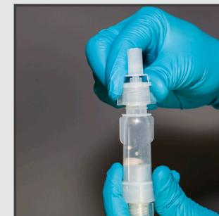
> Screw the injection cap onto the other side of the adsorbent tube.
