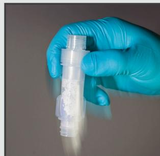
> Mix the lysed sample with the powder in the adsorbent tube by shaking thoroughly.
