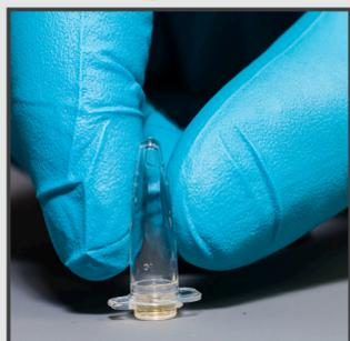
> Incubate the tube upside down for 2 min (use timer) at room temperature to reconstitute the reagents in the cap.
