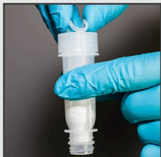
> Remove the cap of the adsorbent tube but do not discard it.
