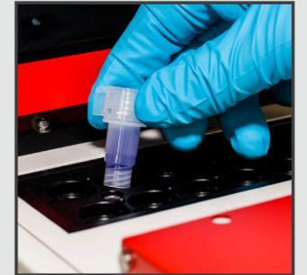
> Incubate the tube in the HumaLoop T heating unit at 90°C for 5 min.
