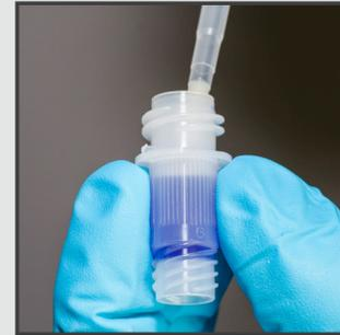
> Transfer the sample slowly into the heating tube. Slowly rinse the tip once to remove the sputum.
