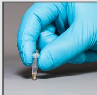
> Flick down the reaction tube until the reaction mixture is collected at the bottom.
