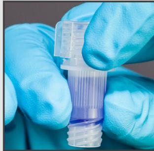
> Remove the cap to open the heating tube of the Loopamp™ PURE DNA Extraction Kit.
