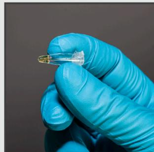
> Mix the contents of the tube by inverting five times.
